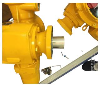
Some valves have no flange at all onto which the actuator can be mounted. In those circumstances, a plate has to be utilized, such as a saddle bracket.
